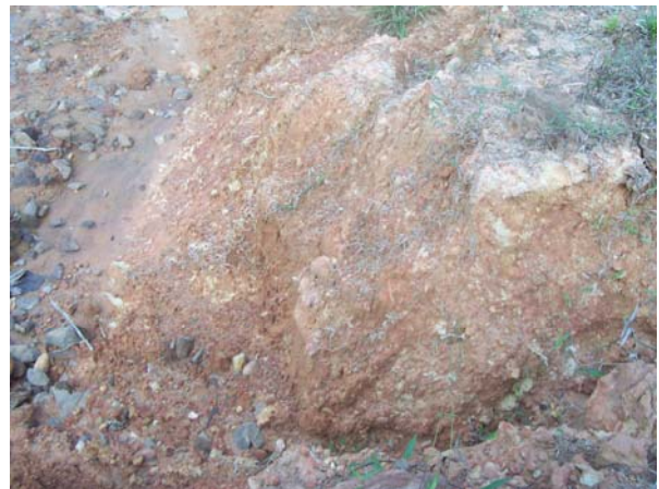
Photo 12: Highly weathered gneiss converted in to clay particles.
